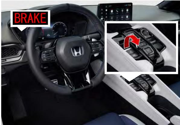
2. Set parking brake by pulling the parking brake switch (P)
