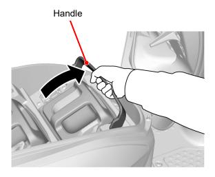
2. Pull out the battery for motor.
