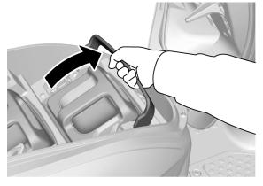
2. Pull out the battery for motor.
