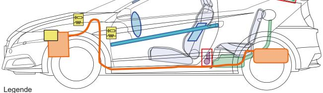
Structural Airbag ≱Ѣ Control unit reinforcements 12 Volt-Gas-Gas filled Battery generator spring unit High Voltage Fuel Seat belt component tank tensioner
