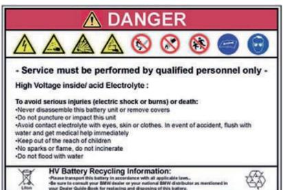
Marking of the remaining highvoltage components:
