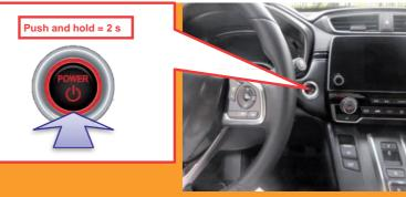
$\frac{Shut down procedure 1:}{Push and hold = 2s}$ Up to 5 min after deactivation still high voltage on system.
